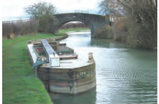
A British Waterways dumb barge with a balance beam for a lock on board
